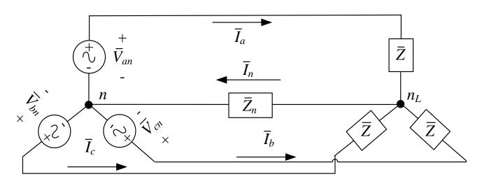
$$\overline{V}_{an} = \overline{I}_{a}\overline{Z} + \overline{I}_{n}\overline{Z}_{n}$$
