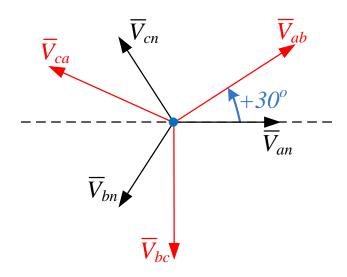
$$\begin{cases} \overline{V}_{ab} = \sqrt{3}V_{\phi} \angle 30^{o} \\ \overline{V}_{bc} = \sqrt{3}V_{\phi} \angle -90^{o} \\ \overline{V}_{ca} = \sqrt{3}V_{\phi} \angle +150^{o} \end{cases}$$
